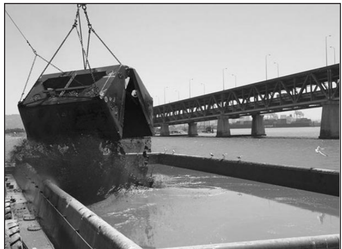
Dredge sediment that is removed from waterways to maintain the navigability of the waters is often laced with toxic chemicals. Photo credit: www.newbaybridge.org
